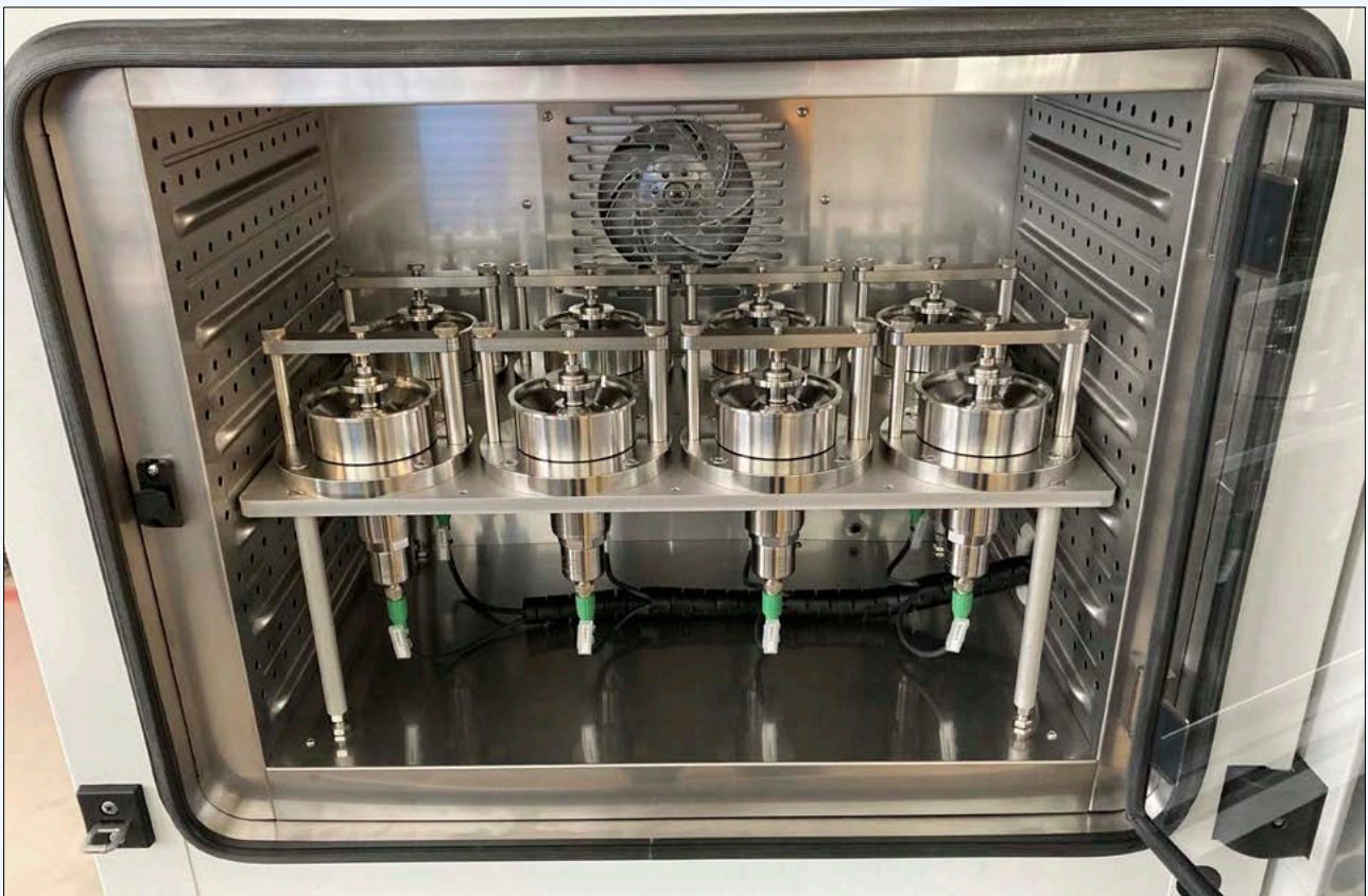
Test cells of the test bench for real-time measurement of the resistance of protective clothing against chemical warfare agents (liquid mustard).
