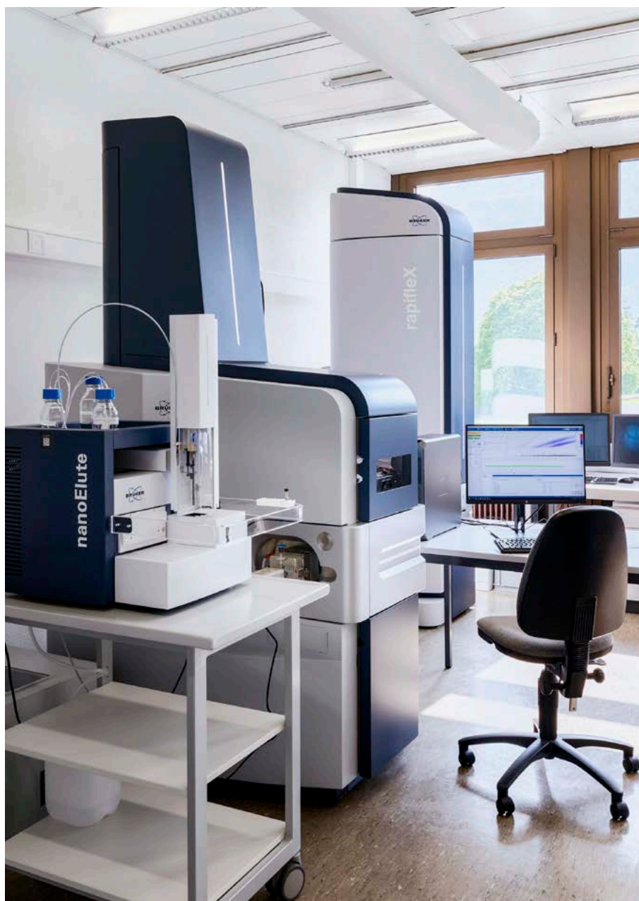
The nano-LC-IMS-QTOF for the detection and identification of toxins
