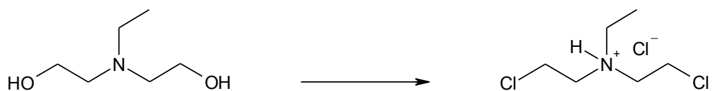
Fig. 9: Schematic presentation of bis(2-chloroethyl) ethylamine synthesis.
