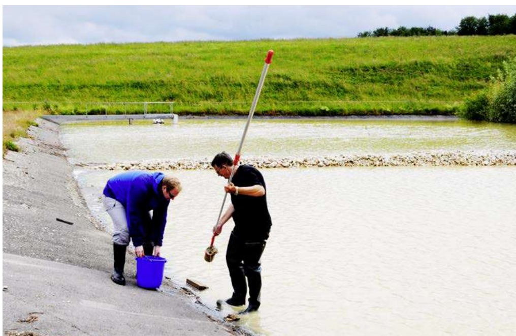
Taking a sample from a sedimentation tank
