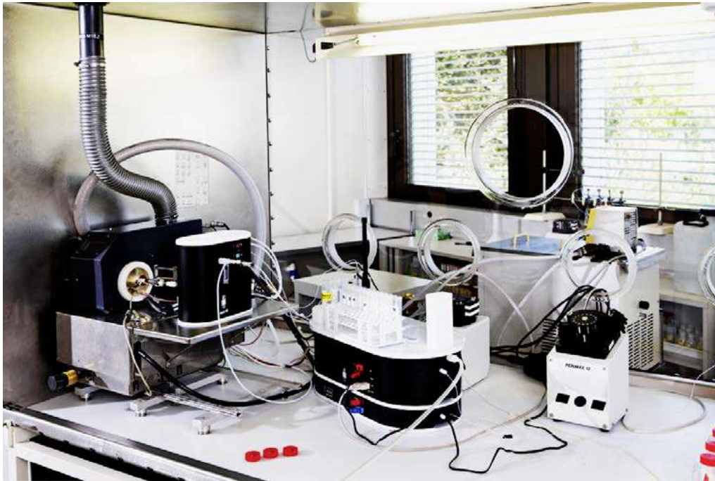
Inductively coupled plasma mass spectrometry (ICP-MS) in Spiez. This method enables high-precision isotope analysis
