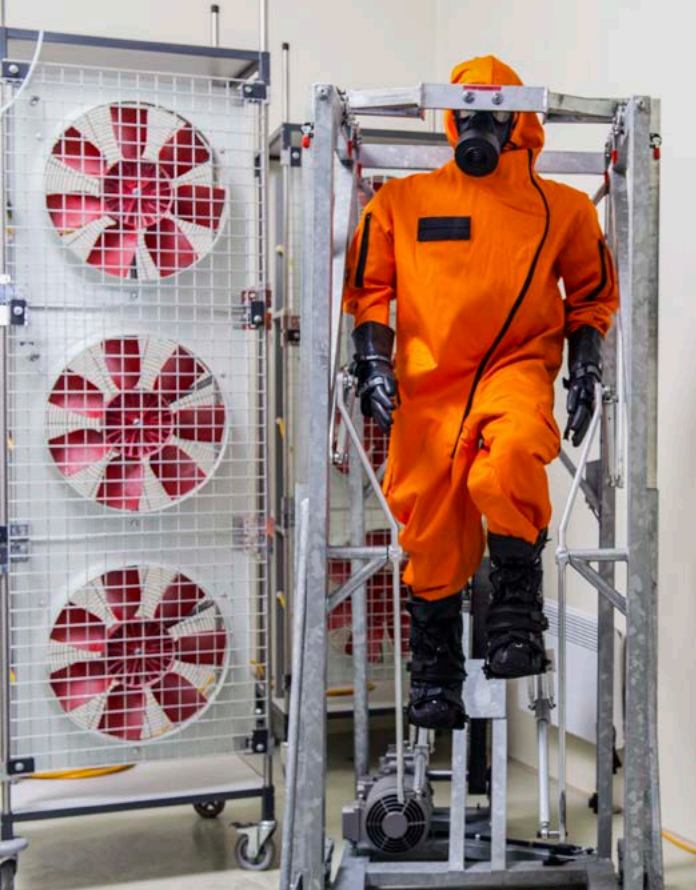
Figure 1: Left: MIST Chamber with wind simulation and moving mannequin at Spiez Laboratory, right: location of the 33 samplers.
