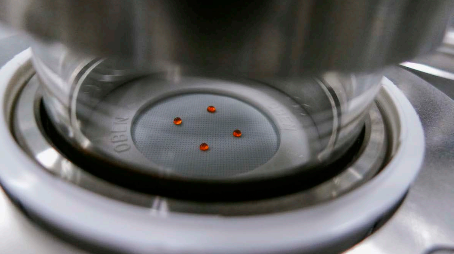
Figure 2: Test material contaminated with 4 \times 4 \mu\text{l} sulfur mustard
