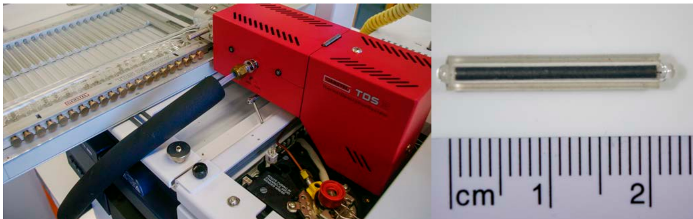
Figure 2 right: Twister® and left: Thermal desorption unit coupled with GC-MS at Spiez Laboratory
