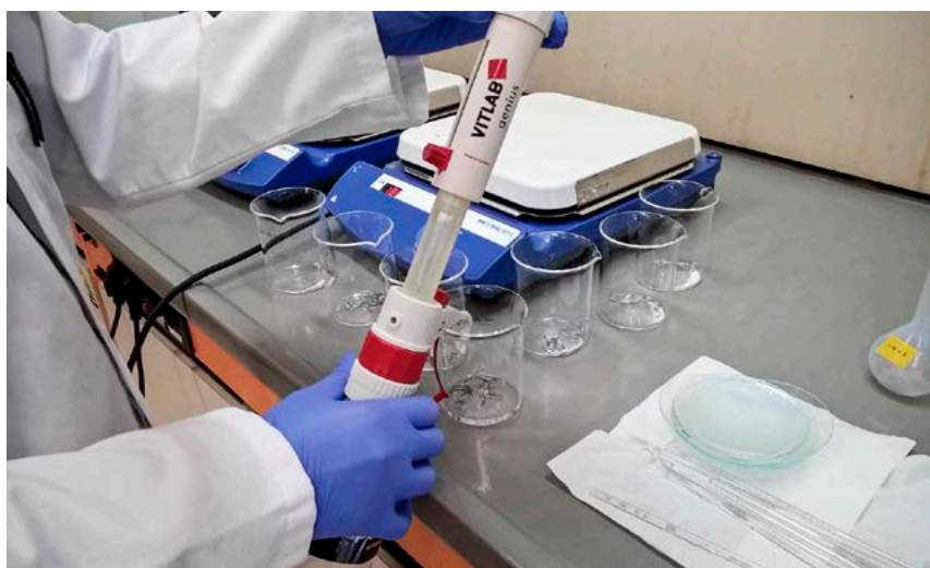
Figure 2: Addition of high-purity nitric acid to the Lead samples in quartz vessels
