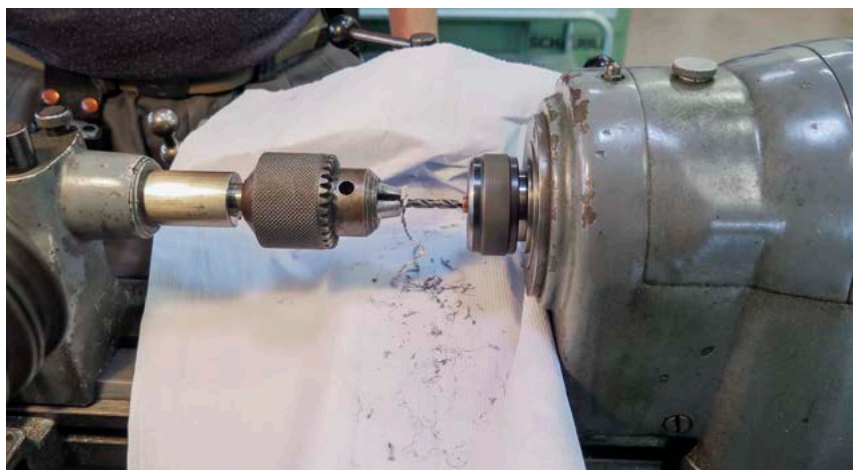
Figure 1: Machining of the Lead specimen
