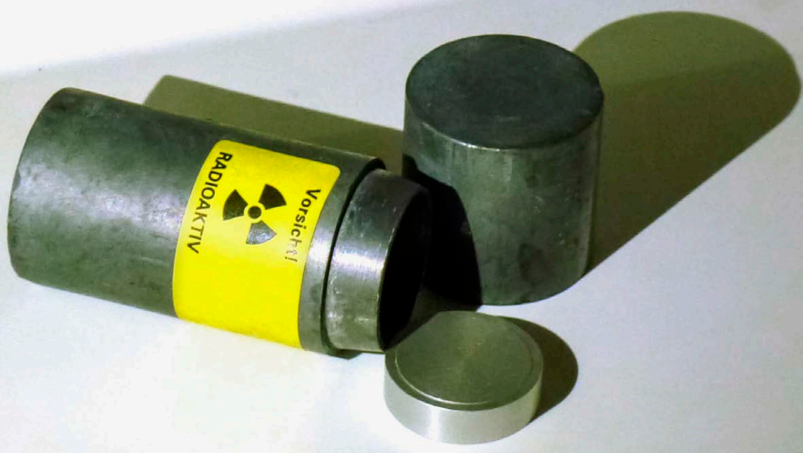
Lead container for shielding radioactive material
