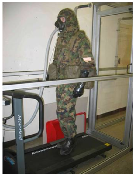
Proband on treadmill in the test chamber
